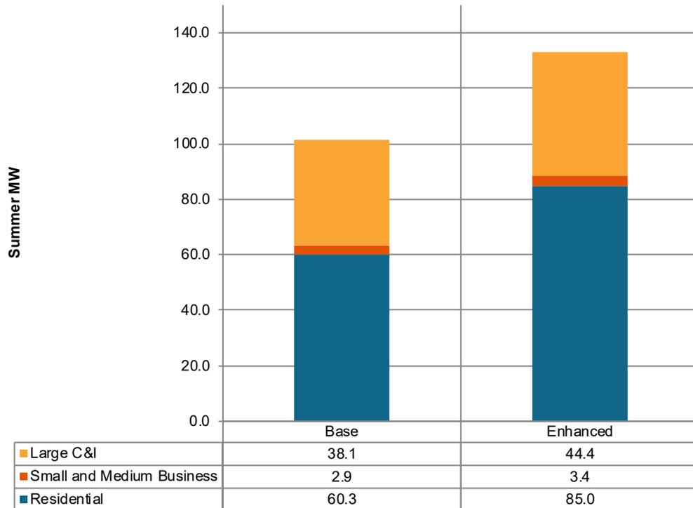
The estimated summer peak capacity is 101.3 megawatts for the base case, and the enhanced case shows expected increases to 132.8 megawatts from increasing program incentive offers over the levels presented in the base case.
