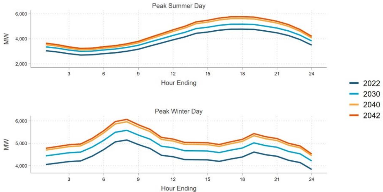
Several patterns are apparent from examining the figure above. First and foremost, forecasted loads shapes are relatively unchanged over time as the total magnitude of projected load increases. Winter peak loads are higher than summer peak loads. The peak hour in summer is typically hour-ending 17:00 and the peak hour in winter is hour-ending 08:00. This potential study therefore focuses on the current summer peak hour, 17:00, and the current winter peak hour, 08:00.
